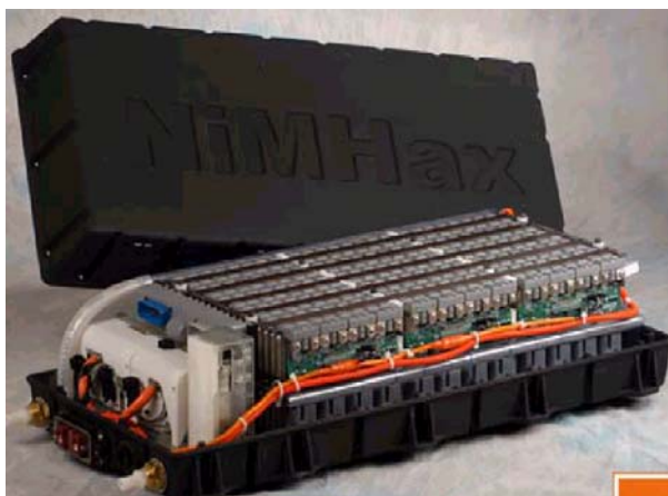
Figure 4.3.6: Nickel-Metal hydride full pack.
